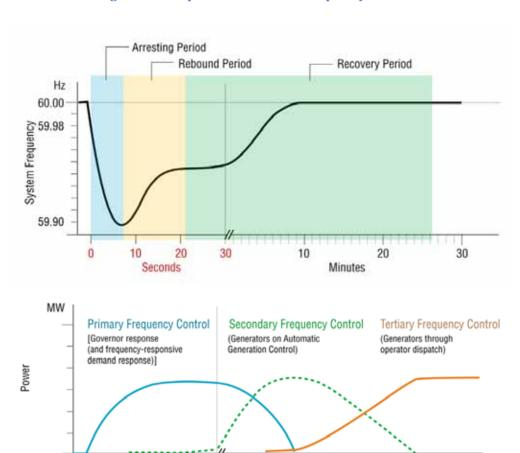
Figure 11 - Sequential Actions of Frequency Controls
