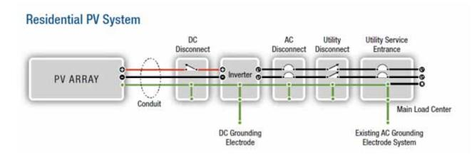
Figure 16 - Residential PV System Schematic
