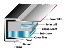
One typical flat-plate module design uses a substrate of metal, glass, or plastic to provide structural support in the back; an encapsulant material to protect the cells; and a transparent cover of plastic or glass. Source: NREL
