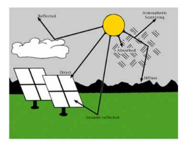
Illustration of the direct solar radiation and the indirect, diffuse radiation that contribute to a PV array. Source: NREL
