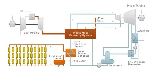
Figure 26 - Solar CSP Hybrid with Natural Gas Co-Firing
