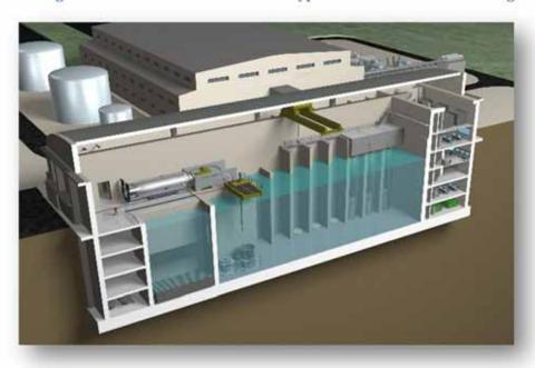
Figure 31 - NuScale Cross-section of Typical NuScale Reactor Building
