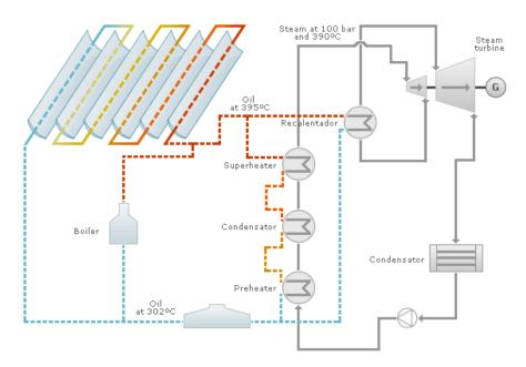
Figure 24 - Solar PTPP Schematic
