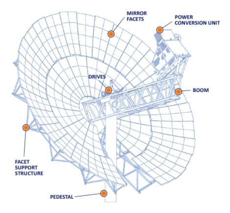
Figure 20 - Stirling Engine Dish
