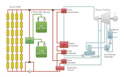
Figure 27 - Solar CSP with Thermal Storage
