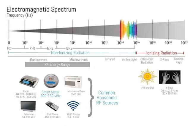
Figure 1. Electromagnetic Spectrum and RF Sources
