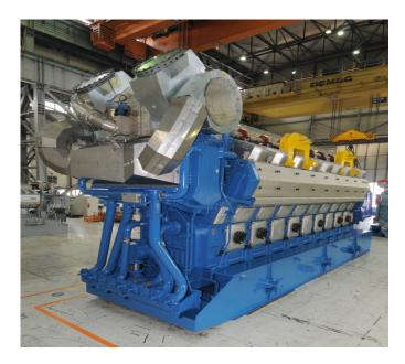
Picture 1 - Wärtsilä 18V50SG engines to be installed at the Sundt Generating Station
